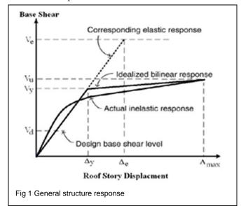
A structure's mathematical model is required for the design and their performance evaluation. In this particular study program SAP2000 is used to perform both linear elastic analysis and non-linear static analysis (pushover) for capacity evaluation of the individual systems.
