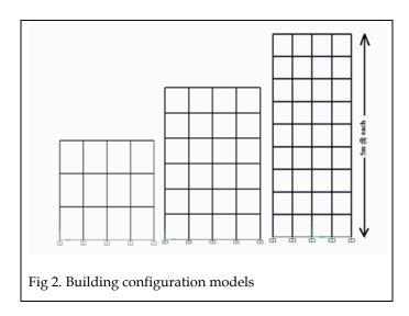
The frames are assumed to be located in seismic zone IV, the soil type chosen is medium and the importance factor assumed is 1. IS 875 part 1 (1987) is used to calculate the dead and live load and lateral loads are calculated as per IS 1893 (2002). The grade of steel used in the present study is Fe250. The live load is taken as 3.5 kN/m2 for floors and 1.5 kN/m2 for roof. Here slab of M25 and secondary beam of I section supporting them are provided.
